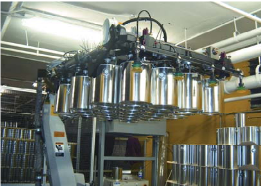
The robot's end effectors pick up half the cans in a pallet stack layer and loads them onto the fill station conveyor (center, behind the lifted cans). The yellow and green suction cups are used to remove the "picture frame" and slip sheets.
